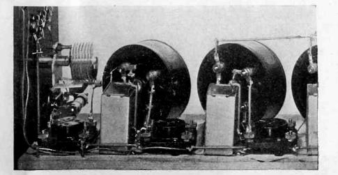
ient because, once set, it requires no further attention. Below, details of the sub-panel and middle deck parts, showing the loop tipjacks, grid leak and condenser, and the bypass condensers. These play a vital part in quality reproduction
