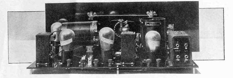
could be accepted by the set builder as the official design, and the safest one to follow. In the wiring instructions and diagrams which accompany this article, the full constructional details of the new Browning-Drake design are given for the first time.
