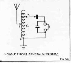
Fig. 32. The historic double-slide tuner circuit, not so long ago the pinnacle of radio achievement
