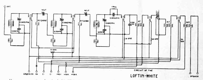
Here are connections for the Loftin-White kit, a new outfit employing a constant-efficiency system which is meeting with a most favorable reception. All parts are of standard manufacture. For further data, write the Circuit Editor of Radio Mechanics
