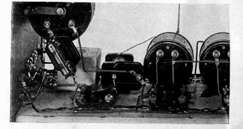
may not be clear in the assembly instructions. Below, a closeup of the lower left corner. Note the arrangement of the grid leak and condenser mounted on the R. F. choke, and the twisted leads from the filament of the power tube to the A. C. binding posts
