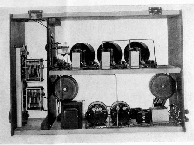
speaker. All the interacting R. F. currents are kept in their places, with the result that the output is clear of undertone noises which would otherwise spoil the quality. This also makes the tuning less critical.
