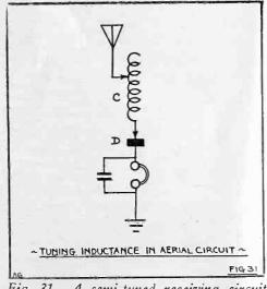
Fig. 31. A semi-tuned receiving circuit
