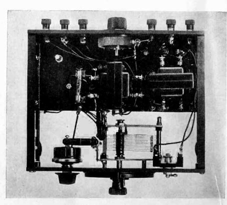
system of regeneration control. This allows the rotating coil, designed as the tickler, to be used for the antenna. Broad tuning is o b t a in e d when the winding on the rotor is parallel with the stator winding. Turning the coil sharpens the tuning, making the set well suited for reception in conjested centers
