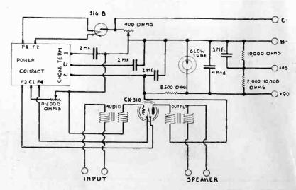
on the 310 socket to P on the output transformer, and connect F and G to tip jacks L.S. 1 and L.S. 2.
