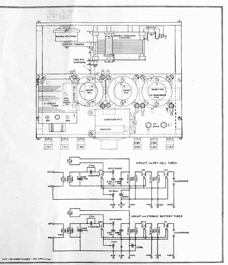
Connect 3, on the stator of the variable condenser, to the lower right hand terminal of the coil, going to the secondary, and connect it also to the forward lug on the grid condenser.
