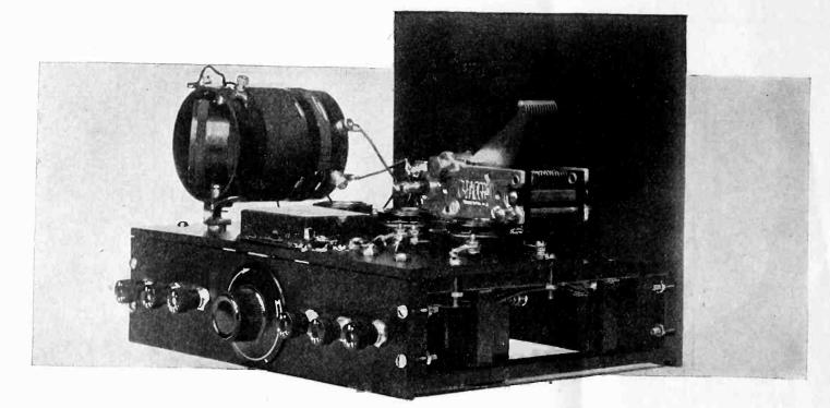
latter for DX. If you use dry cells, you should measure the voltage across the filament terminal, from F—on socket No. 1 to the A—BAT binding post. This should show exactly 6 volts for the 199 and 120 combination. Do not use more voltage than that.
